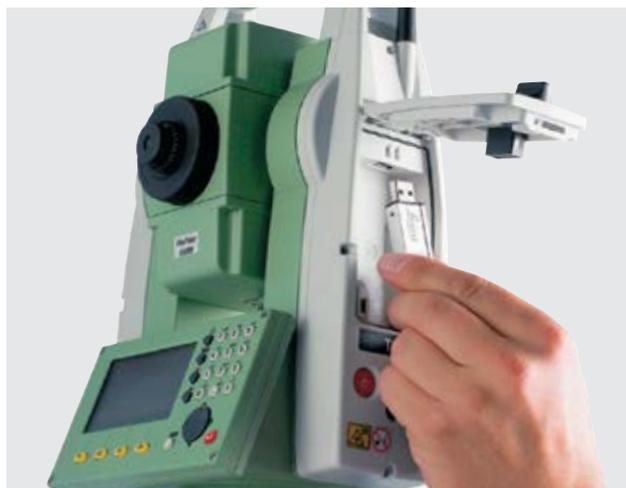
The Leica FlexLine TS06plus communication side cover enables cable-free connection to any data collector via Bluetooth®, for example the field-controllers Leica CS20 controller or Leica CS35 tablet with Captivate software. The USB-stick enables the flexible transfer of such data as GSI, DXF, ASCII, LandXML and CSV.
