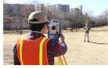
**Easy "TOPO" operation** Just "Rough Aim" and "Press Trigger button" to get precise aiming and measurement to prism target.
