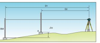
• Setting-Out Measurement The SDL50 can perform setting-out measurements in three ways: by height difference, elevation and horizontal distance.
