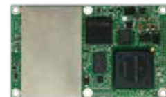
Advanced BD970 OEM is a compact multi-constellation receiver designed to deliver centimeter accuracy to a variety of applications.
